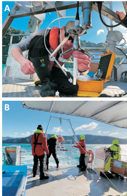
Figure 3: (A) The measuring head of the eddy-covariance lander consists of an acoustic doppler velocimeter and an oxygen sensor (micro-optode). This device provides a non-invasive measurement of the sediment oxygen consumption. (B) To test deployment and measurement protocols, the project team co-deployed both landers, the eddy-covariance and the chamber lander, in 82 m water depth off the coast of New Zealand.
