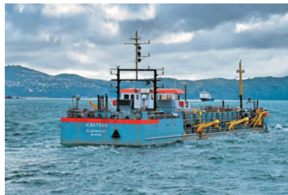
Dredging vessel The Albatros operating in the Wellington Harbour entrance, removing 30,000 cubic metres of sand build up from critical shipping channels, 23 April 2021 (Photo: CentrePort).
