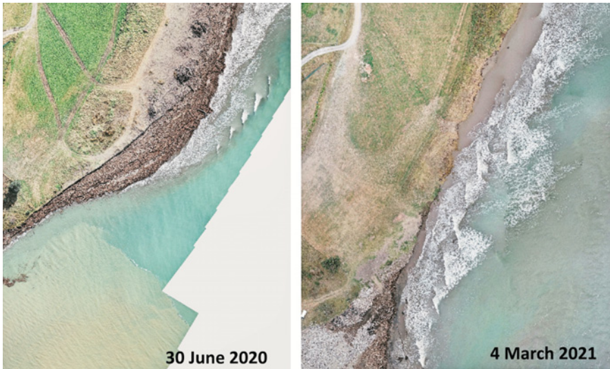
Figure 6: Drone Maps of the mouth of the Uawa River 30th June 2020 showing the scour associated with a major river flood the previous week (left) and the same area in March 2021 showing erosion of the shoreface north of the river mouth (right).
