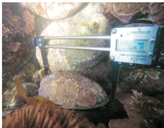
Measuring pāua during biomass estimates using underwater electronic callipers. Pāua that have been measured are marked with a yellow crayon so they are not re-counted during that survey (Photo: Tom McCowan).
