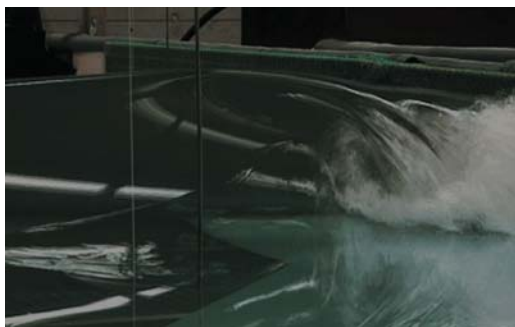
Figure 3: Physical modelling of waves in the ASR laboratory. Courtesy ASR Ltd.
