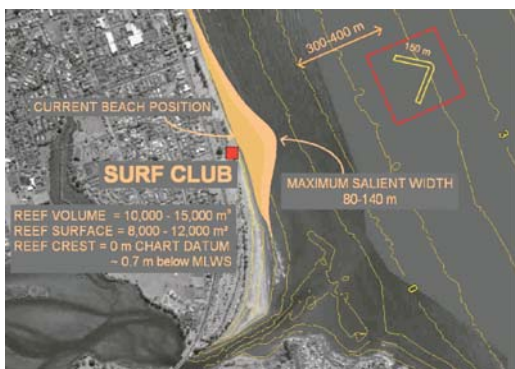
Figure 4: Feasibility study showing a desired beach response to a reef placed just north of the surf club. Courtesy OBRCT.
