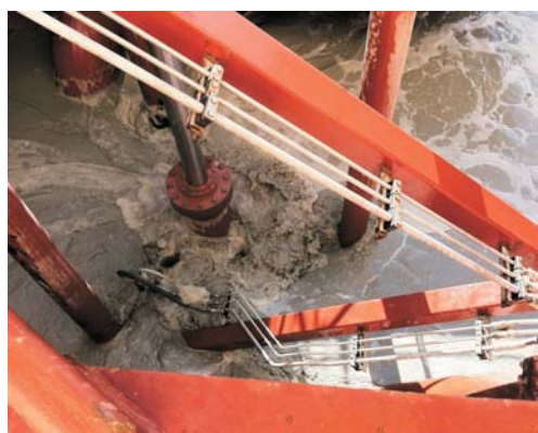
Image shows the structure of the discharge funnel from the hopper including the “green” or environmental valve. The purpose of the valve is to reduce the amount of air being discharged with the sediment, allowing the sediment to sink to the seabed faster, which reduces turbidity. Image: Willem de Lange.
