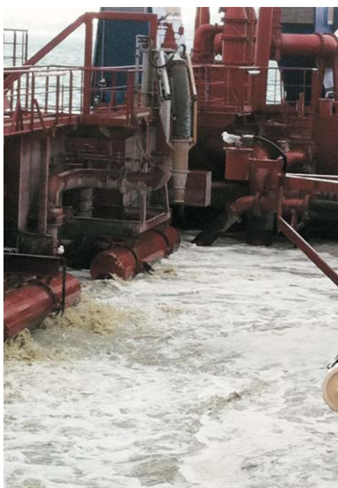
(Top image) This image shows the entrainment of air, which creates bubbles. At the top is an adjustable funnel that can be released and lowered to vary the rate of discharge, which also reduces the turbidity. Photo: Willem de Lange.
