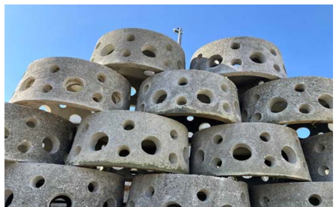
Figure 2: Sea Nests being poured and stored at McGregors Concrete yard (Photo: Waka Miller, Sea Nest Ltd).
