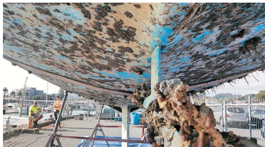
The hull of the SV Wahoo prior to cleaning and antifouling treatment (Photo: Phillip Karaitiana).
