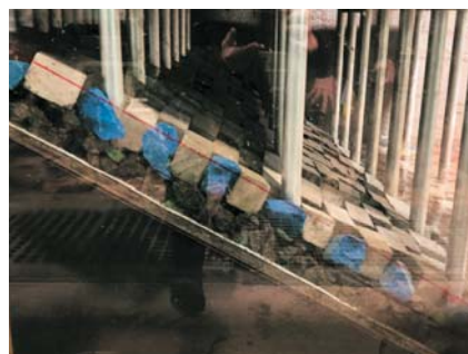
Figure 7: Wave tank testing at the UNSW Water Research Laboratory (Australia) for the specially-placed precast concrete block revetment (side view).
