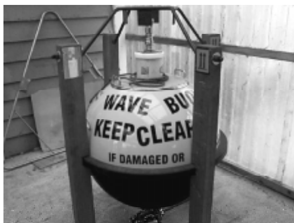
Figure 1: Wave buoy following painting and preparation (note packing case)
