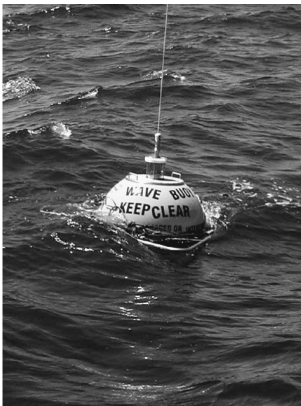
Figure 2: Wave buoy shortly after deployment
