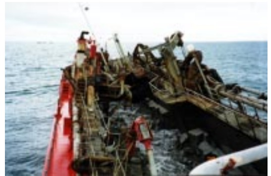
The Pelican's split-hull opening and dropping its load of sand to the seabed
