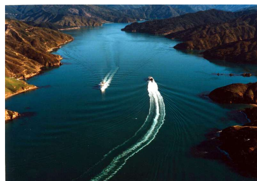
Figure 1: A conventional ferry travelling at sub-critical speed on the left and a fast ferry travelling at super-critical speed, in Tory Channel (© Marlborough District Council, used with permission. Graeme Matthews, Photographer)
