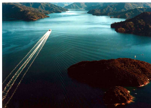
Figure 2: A fast ferry travelling at close to critical speed (© Marlborough District Council, used with permission. Graeme Matthews, Photographer)
