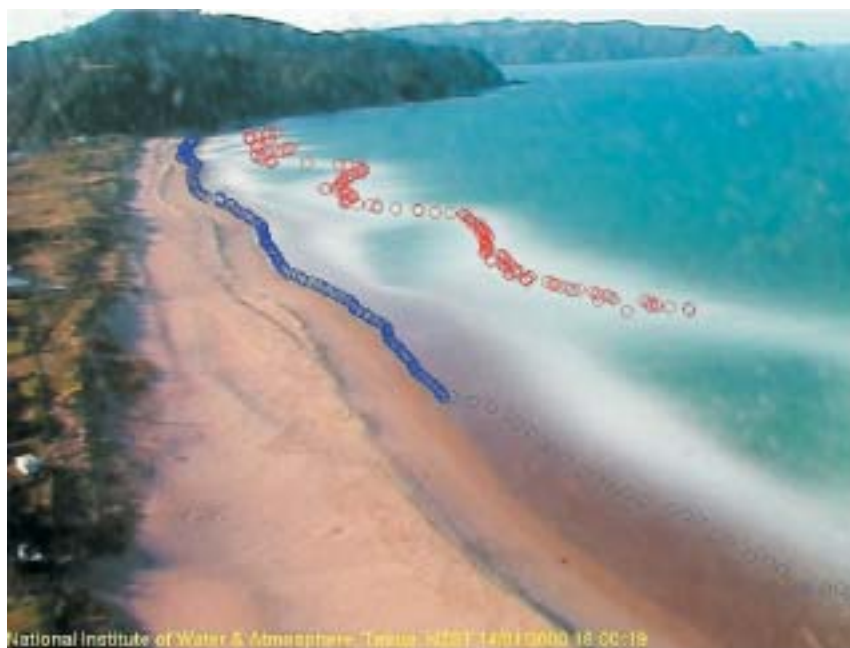
Figure 2: The 10-minutes averaged image allows detection of sandbar (seaward circles) and shoreline (shoreward circles). The sandbar location is assumed to correspond to the location of maximum wave breaking intensity while the shoreline is detected using an algorithm that captures the difference between the sand and white foam associated with the wave run-up.
