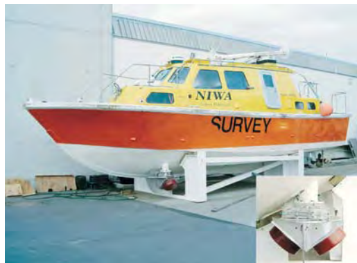
Figure 1: Hull mounted EM3000D multibeam system on survey launch Pelrous.
