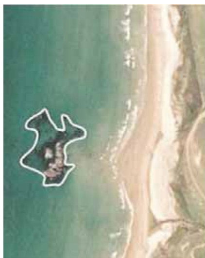
Figure 3: Natural coastal protection (a salient) formation in the lee of a submerged reef at Opito Bay, Coromandel (left). Sediment evolution modelling was used to simulate the formation of the salient at Opito Bay. RTK surveys of the bathymetry and beach were used to first calibrate and then verify the modelling (right).
