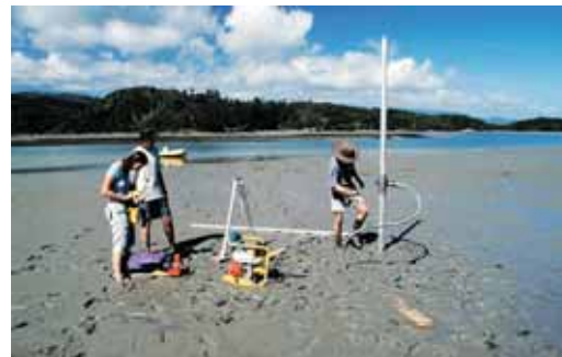
Figure 2: Vibrocoring on the sand and mud flats in Whanganui (Westhaven) Inlet.
