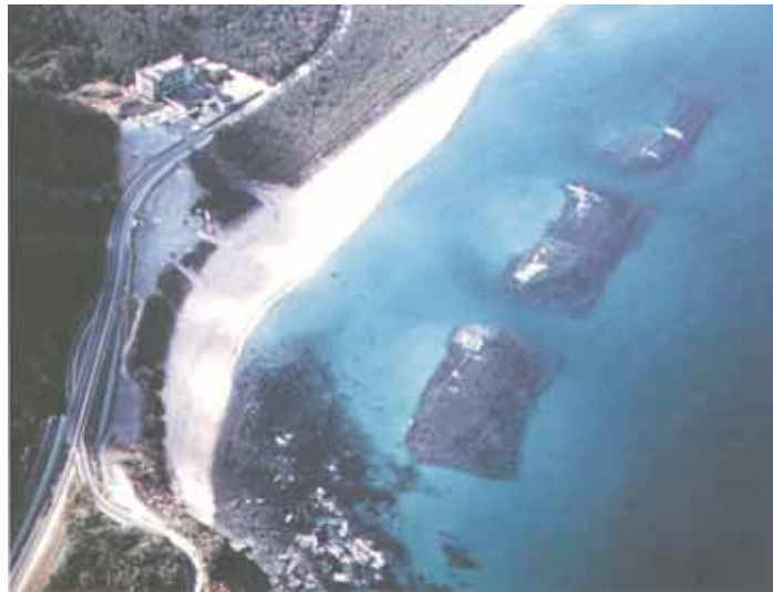
Figure 2: Simple submerged reefs used for coastal protection in Japan. The similarity with the St Claire, Dunedin, situation is striking - with a thorough understanding of the site and incorporation of surfing amenity to mitigate where it already exists, submerged reefs could be a viable option to retain beach sand at the western end of St Claire.
