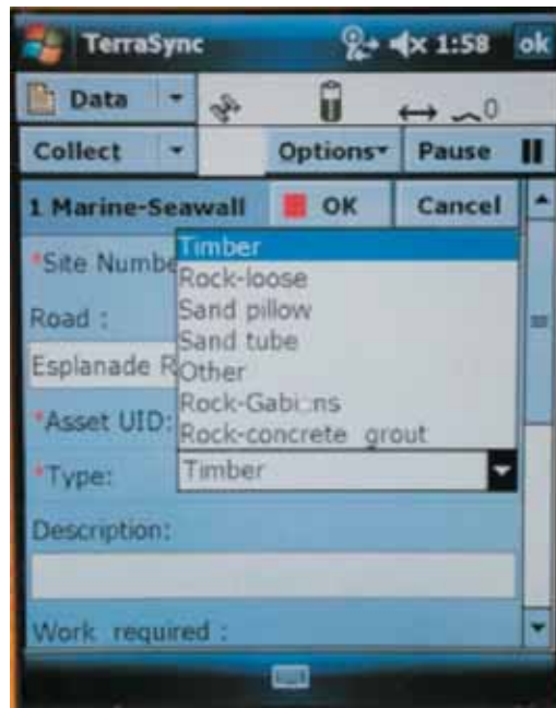
Figure 1: Example of the customised data entry form used to collect condition assessment information within the handheld GPS.
