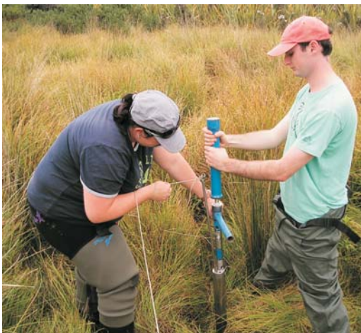
Figure 1: Taking a sediment core
