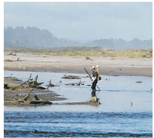
Figure 4: GNSS survey of Totara Lagoon
