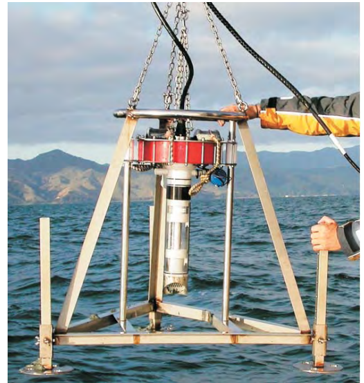
Figure 1: The SPI-Scan instrument used to obtain high-resolution in situ sediment profile images.
