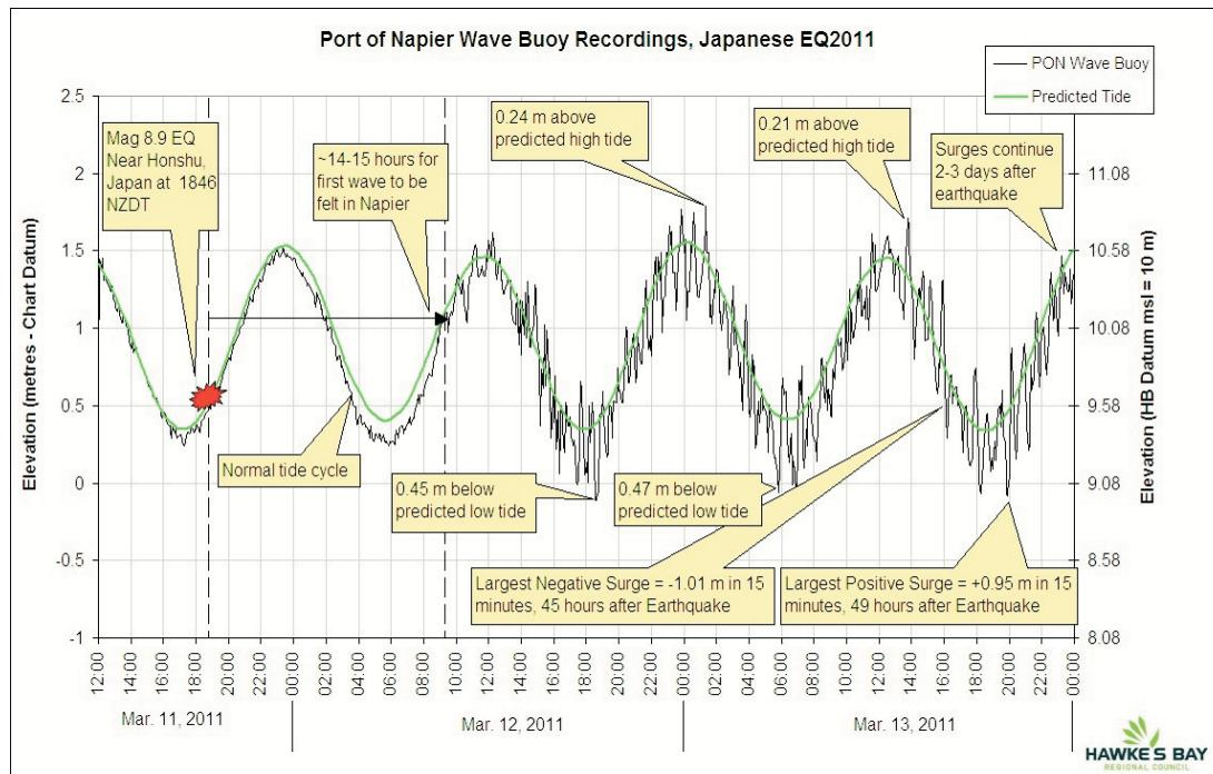
Tide vs Wave Buoy Recordings, Port of Napier.
