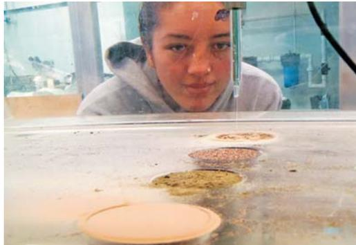
Figure 1: Researcher Aysha Hohaia checks on a working section of a seawater flume that has four inserted sediment cores and a microelectrode in place to measure pH and oxygen pore water profiles. The surfaces of the first and fourth sediment cores have been treated with terrestrial clay.
