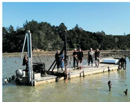
Figure 2: Waikare Inlet oyster farmers trial a barge and hydraulic arm for removing waste timber. Photo: Northland Regional Council.
