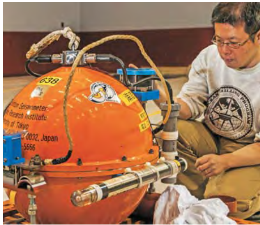
Dr Kimi Mochizuki of the University of Tokyo prepares one of the ocean bottom seismometers prior to deploying on the seafloor off Poverty Bay. Photo: Margaret Low, GNS Science.
