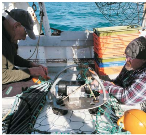
Attaching a camera to a net to study fish behaviour, Gisborne, 2014.
