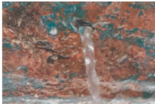
Water leaking from the hull of the unsafe vessel that was removed from Tairua Harbour.
