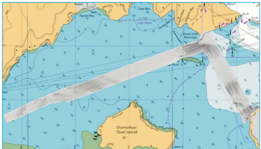
Figure 1: Seafloor reflectivity generated by the Geoswath Plus multibeam system. The mosaic uses a grid-cell size of 0.4 m. High reflectivity is indicated in dark grey, low reflectivity in light grey.
