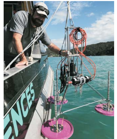
Figure 4: Evan Brown, a member of the AUT marine research group, deploys an automated sediment porewater analyser in Man O'War Bay, Waiheke Island, in about 10 m water depth. The robot uses four electrochemical microsensors to resolve microscale changes in pH and oxygen at the sediment–seawater boundary.
