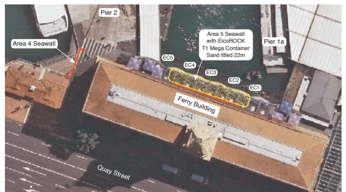
Figure 1: Aerial view of the Auckland Ferry Terminal showing locations of scour areas.
