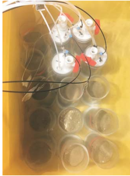
Figure 2: Aquaria within the Ocean Acidification Laboratory at Auckland University of Technology. Sediment cores are collected from Man O’War Bay in the Hauraki Gulf, and exposed to different pH levels in the laboratory, to mimic future ocean acidification scenarios. Shown in the top left cores: sediment oxygen and nutrient consumption rates are measured by carrying out incubations on sealed cores, fitted with oxygen sensors and peristaltic pumps to create water flow throughout the 4-hour incubation period.
