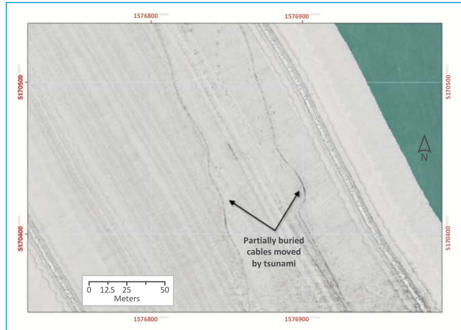
Figure 5: Geoswath backscatter mosaic showing partially-buried and outcropping cables on the seafloor adjacent to Pauahinekotau Head.
