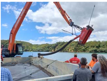
Trial run of the new Johnson Bros dredging tool in Northland (Photo: NRC).
