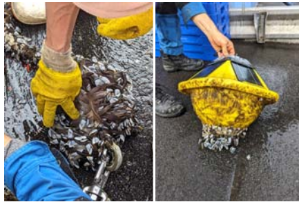
Offshore buoy going for a ride: (left) spotter buoy drifting towards Hawke's Bay shores until the rescue arrival (Plot sourced from Spotter buoy dashboard); (right) biofouling growth after three months of buoy deployment (Photo: João Albuquerque).
