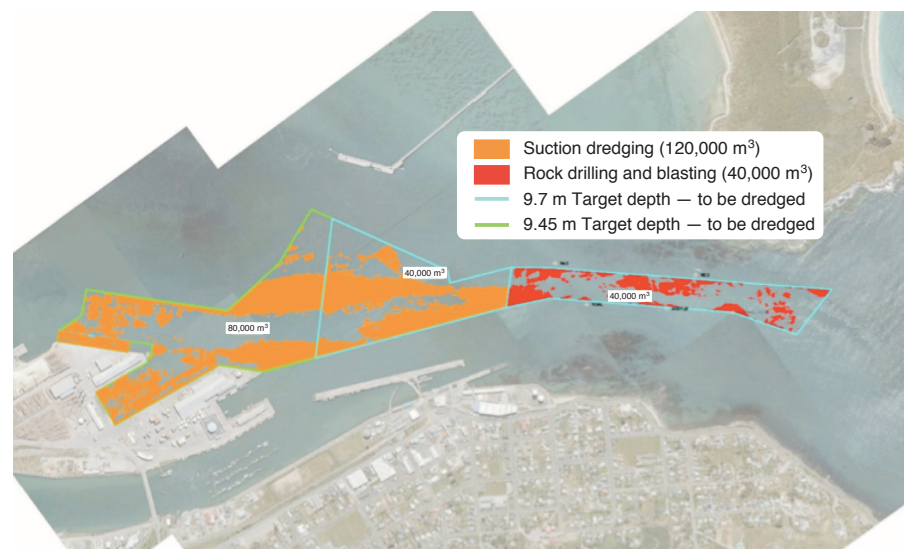
Figure 2: Proposed dredging and blasting locations, Bluff Harbour (South Port NZ Ltd).
